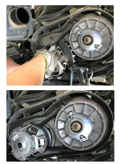
7. Install DURACLUTCH Primary with hardware provided as shown. Tighten bolt to **60 ft-lbs**. **VERY IMPORTANT**- <u>Over</u> tightening will not allow clutch to operate properly and cause damage and failure of the clutch.
