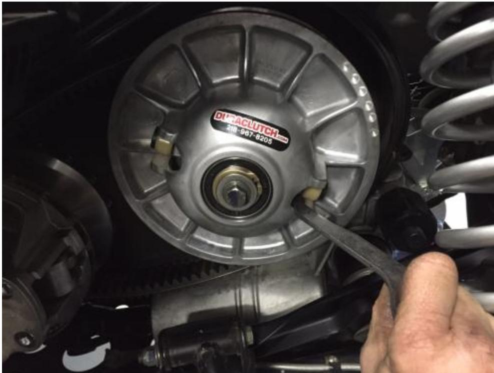
8. Set belt tension. Place transmission in PARK! APPLY FOOT BRAKE TO INSURE VEHICLE REMAINS STATIONARY. Apply slight throttle to turn Secondary.
