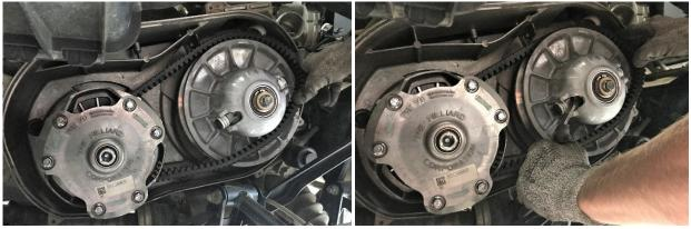
10. Install outer clutch housing.
