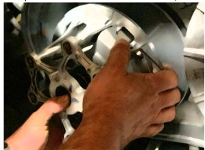
3. Pull the Polaris primary fixed sheave from the engine crankshaft using the 99-012 puller provided.
