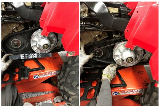
6. Slide belt into DURACLUTCH DCR Primary clutch then install on post. Use stock primary hardware removed in step 4- spacer, washer and lock washer. Tighten bolt to 47 ft-lbf.
