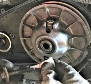
5. Remove Primary clutch bolt. Remove the stock Primary clutch with puller SVI # 25-126. Greasing the end of the puller slightly will aid in removal. Do not get grease on any clutch components.
