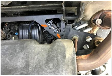
16. Take two 8-inch cable ties and feed thru tab on top of dongle housing and around the frame and tighten
