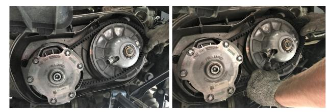
13. Install outer clutch housing. Ensure seal is good or replace.
