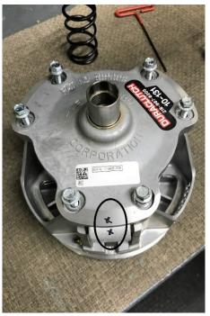
5. Remove weight pins, weight pin nuts, weights and primary spring.
