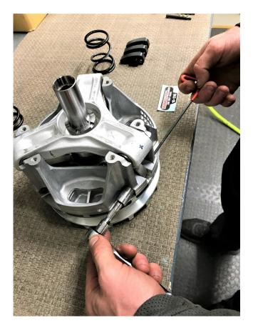
Install new 10-171 RG-75 weights into clutch, install the 3 new weight pins in the same direction and weight pin nuts provided in kit.
