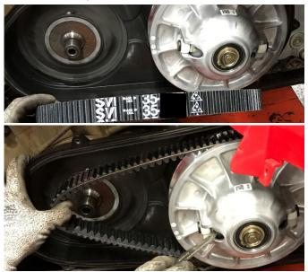
8. Slide belt into DURACLUTCH DCR Primary clutch then install on post. Use stock primary hardware removed in step 5. Tighten bolt to 47 ft-lbs.
