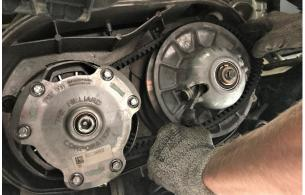
13. Install outer clutch housing. Ensure seal is good or replace.
