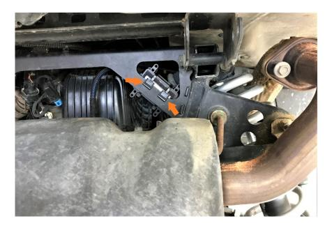
15. Take two 8-inch cable ties and feed thru tab on top of dongle housing and around the frame and tighten.
