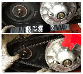
8. Slide belt into DURACLUTCH DCR Primary clutch then install on post. Use stock primary hardware removed in step 5. Tighten bolt to 47 ft-lbs.
