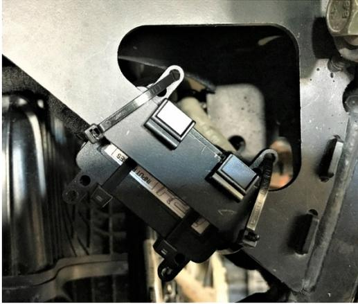
16. Disconnect speed sensor on transmission. Connect end from dongle to transmission. Connect wire removed from transmission into other end of dongle. Make sure Dongle does not interfere with any moving components, such as suspension or shifting assembly. Use remaining cable ties to secure wires as necessary and clip excess tie ends.
