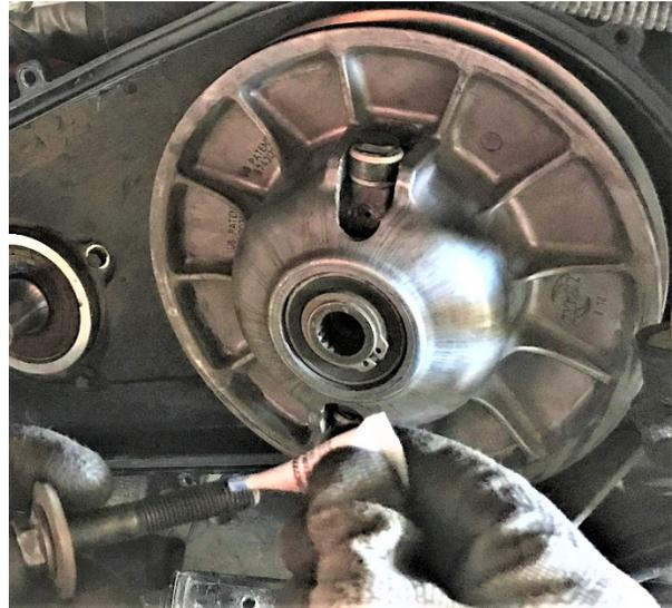
5. Remove Primary clutch bolt. Remove the stock Primary clutch with puller SVI # 25-147. Greasing the end of the puller slightly will aid in removal. Do not get grease on any clutch components.
