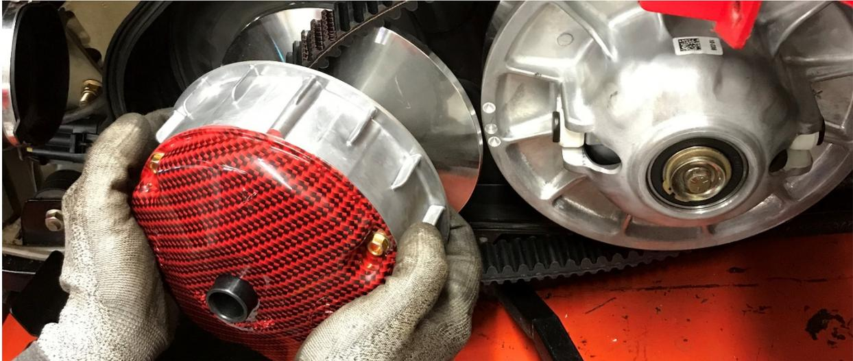
9. Set belt tension. Place transmission in Park and make sure machine is turned off. Rotate secondary by hand to seat belt in secondary clutch until belt tension is tight.
