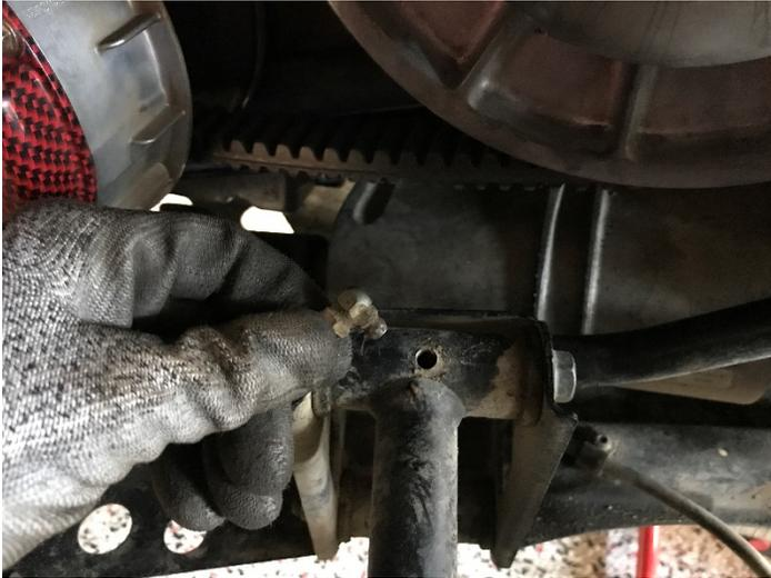
2. Remove stock secondary clutch. Pay attention if there is a snap ring on the shaft and if there are any washers on the shaft with the snap ring. If there is a snap ring or washers remove them. There also may be washers on the spline at the end of the shaft. If there are any remove and discard.
