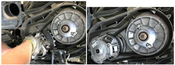
Install DURACLUTCH Primary screw with shoulder washer as shown. <u>DO NOT USE</u> the O.E. flat washer or lock washer. The flat washer will interfere with the primary cover. Tighten bolt to **60 ft-lbs**. **VERY IMPORTANT**- <u>Over tightening will not allow clutch to operate properly and cause damage and failure</u> <u>of the clutch.</u>
