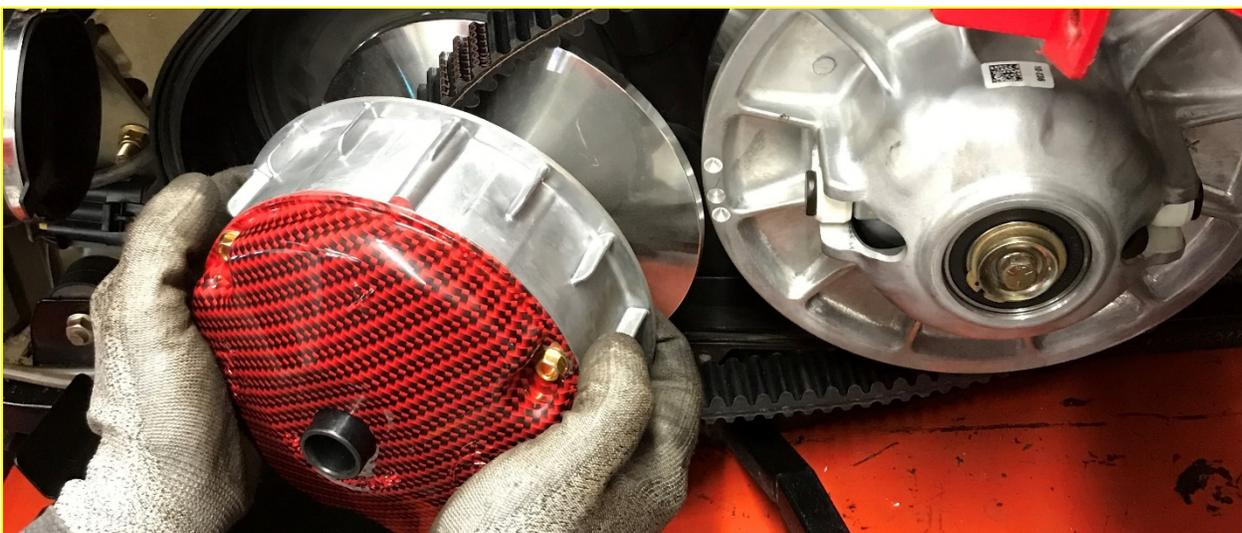
7. Tighten stock primary bolt to **60 ft-lbs. VERY IMPORTANT-** Over tightening will not allow clutch to operate properly and cause damage and failure of the clutch.
