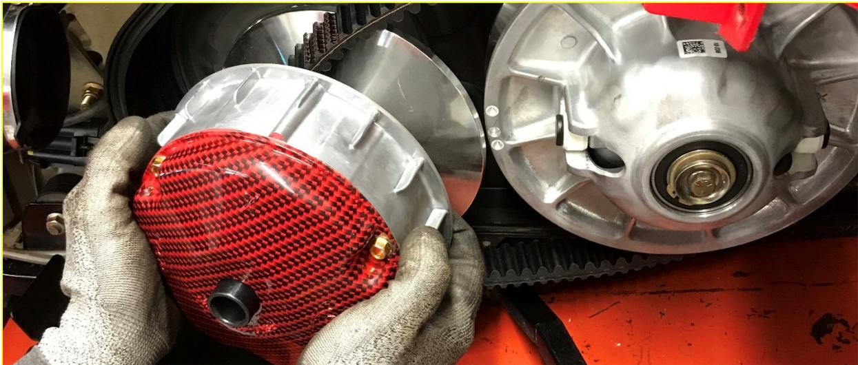
7. Tighten stock primary bolt to **60 ft-lbs. VERY IMPORTANT- Over tightening will not allow clutch to operate properly and cause damage and failure of the clutch.** A 3/8 socket extension can be used to hold primary into one of the outer fins, make sure the extension is seated flat and up against clutch.
